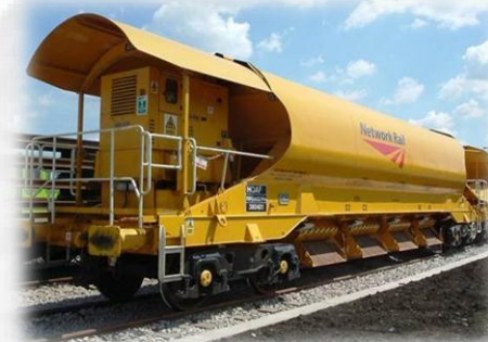
HQA Auto-ballaster 30kVA Air-Cooled set Channel Tunnel Rail Link
