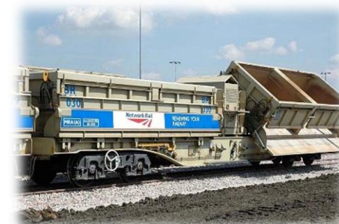
MRA Side-tipper 30kVA water-cooled set Radio-controlled tipping
